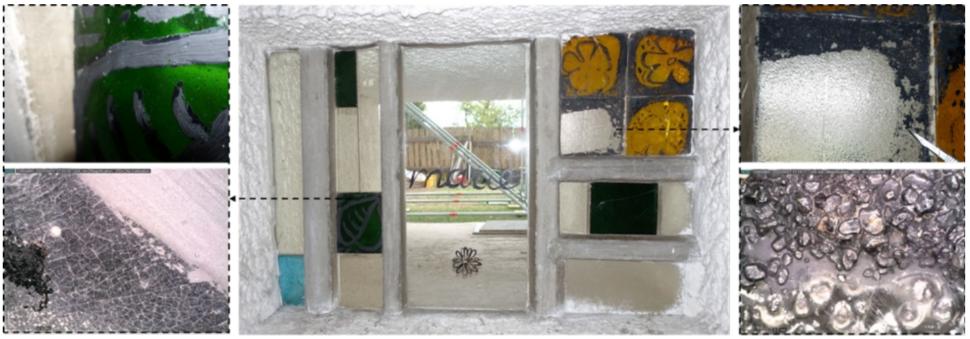
Top left: current architectural polychromes of a Zig-zag house. Right: "direct light" view of a sample for spectrophotometric data sampling. Bottom left: observation of a micro-sample of ultramarine blue under a scanning electron microscope (x160). Photos: CICRP - J. Berthonneau and O. Guillon / © FLC / ADAGP
